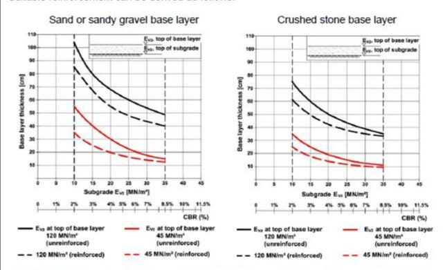
The Y-axis indicates the reduction in the required thickness of the basecourse achieved through the use of Fornit reinforcement.
